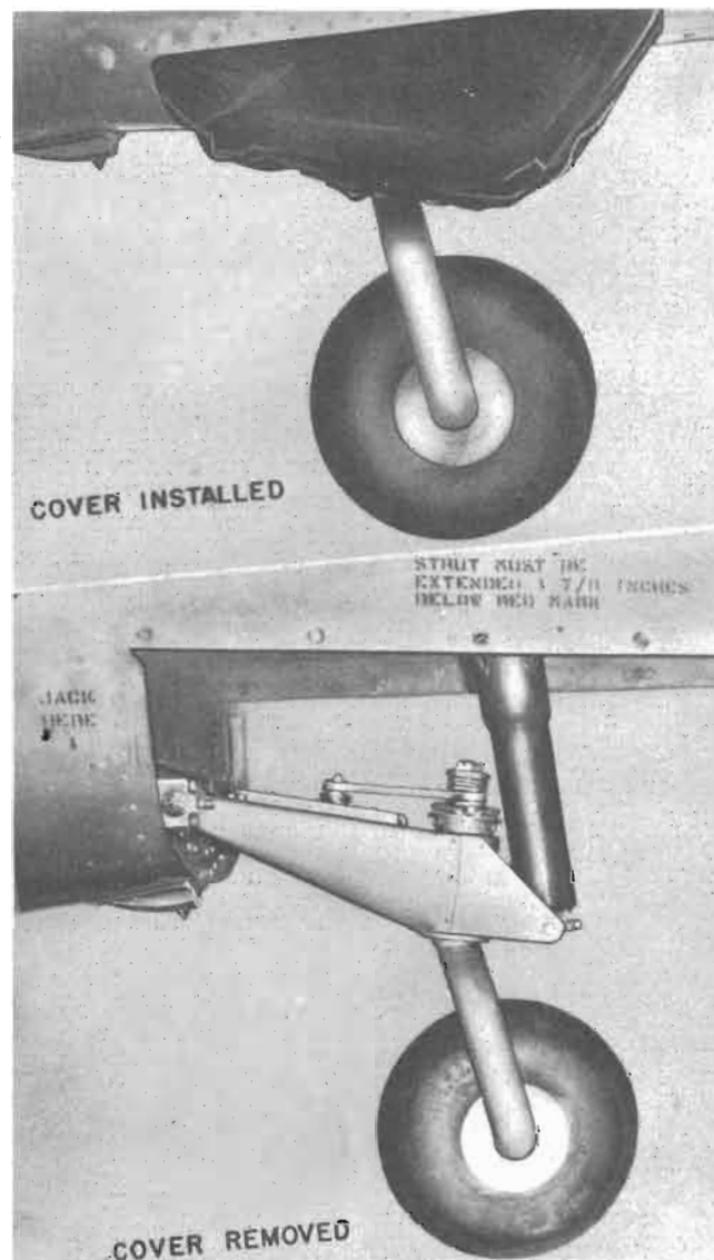
Figure 122 — Tail Wheel Landing Gear Installed
