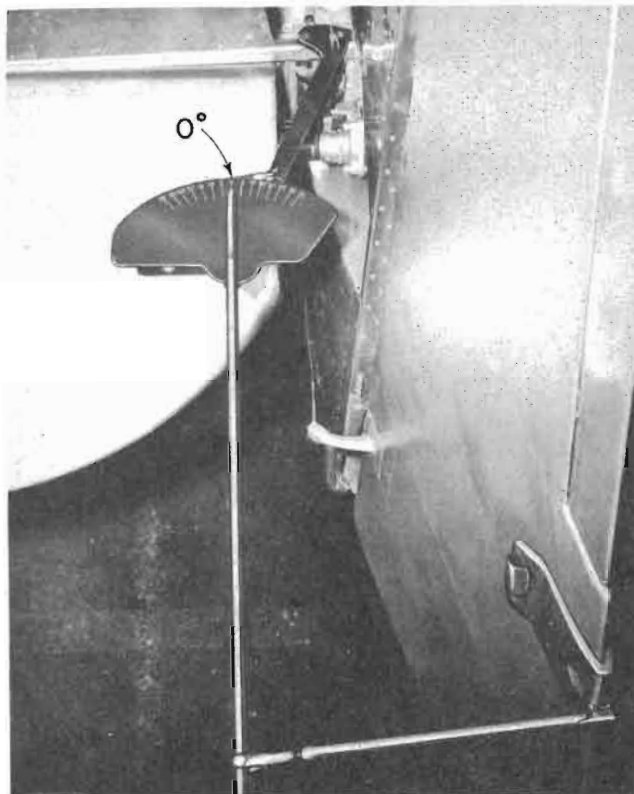
Figure 200 — Checking Rudder Angular Travel (Left and Right)
